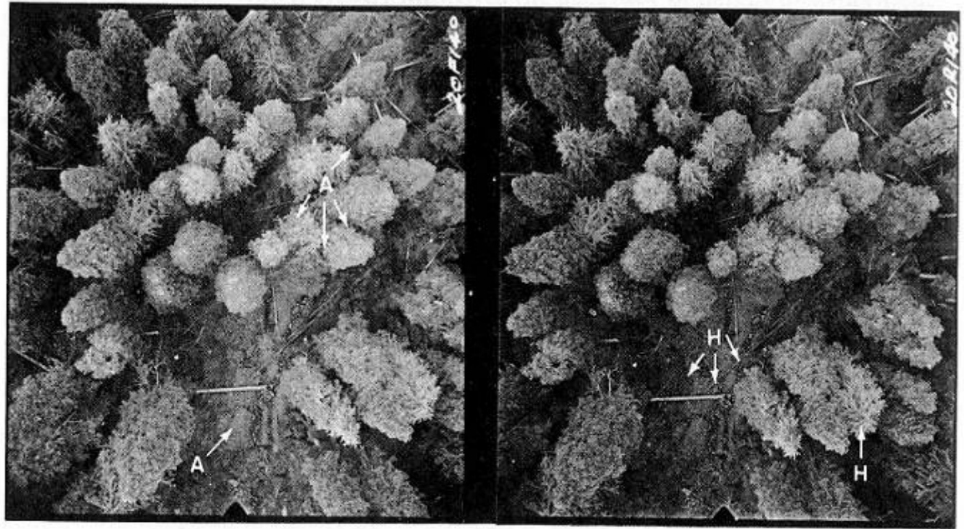
Figure 20.5. Large-scale (PSR = 1364) 70 mm stereogram used for individual tree measurement and species identification in British Columbia. Maximum heights are 150 ft for western hemlock at H and 190 ft for amabilis fir at A . (From E. H. Lyons, 1966, copyright 1966, by the Canadian Institute of Forestry, Quebec, Canada, reproduced with permission, photos courtesy E. H. Lyons.)
